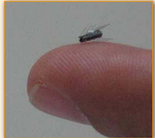
The robot hereby presented has the ability to crawl within cavities with similar characteristics as the typical human body's veins and arteries. The miniaturization achievement is unprecedented, as is the ability to control the robot's activity for an unlimited period of time, for any medical procedure.
